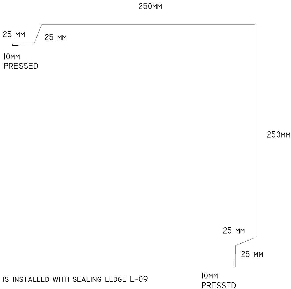
FLASHING IS INSTALLED WITH SEALING LEDGE L-09
