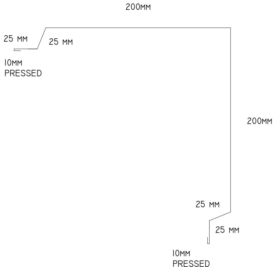
FLASHING IS INSTALLED WITH SEALING LEDGE L-09
