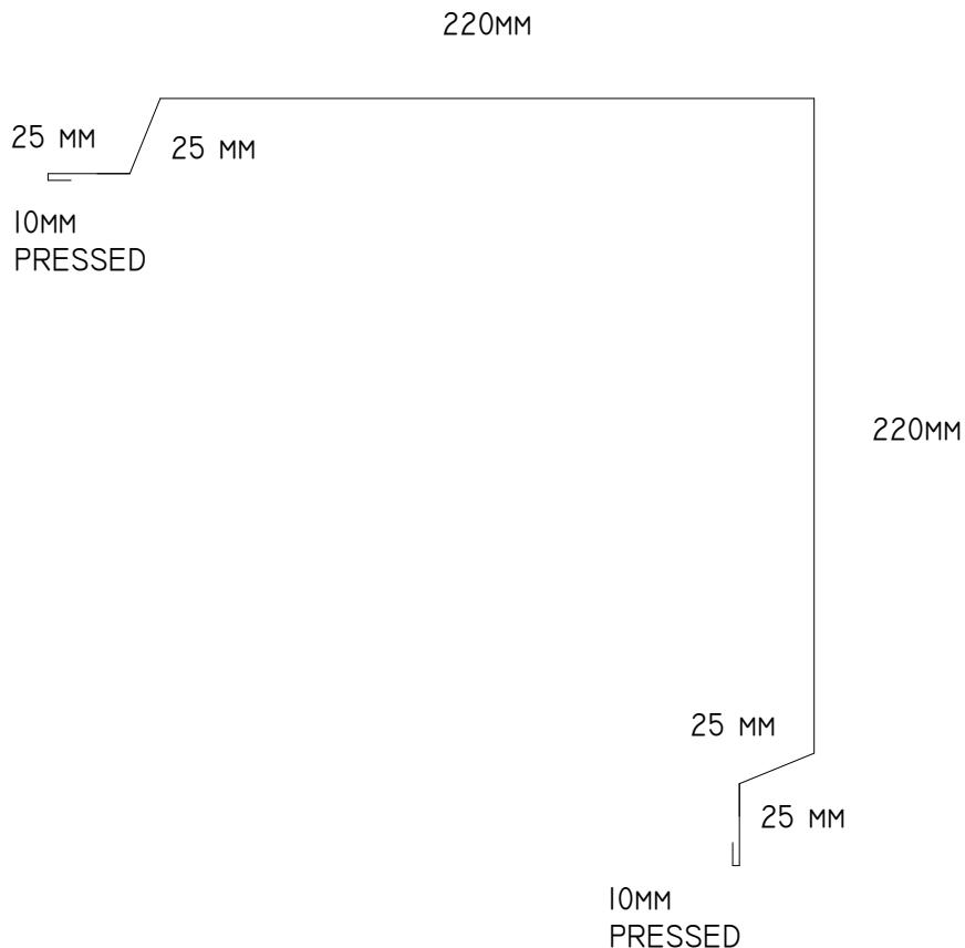
FLASHING IS INSTALLED WITH SEALING LEDGE L-09
